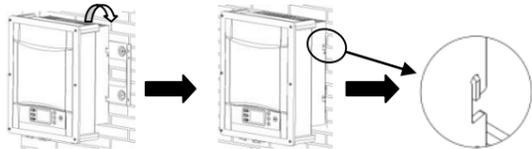
3. Attach the outer fins of heat sink to both sides of the wall bracket using M5 screws(T25 screwdriver, torque: 2.5Nm), as shown in Figure A. If additional grounding or equipotential bonding is required, ground the inverter as shown in Figure B.
